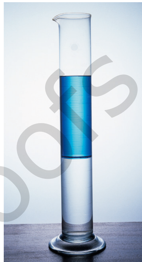
FIGURE 16.4.6 A mixture of paraffin oil (coloured blue) and water (clear) separates into two distinct layers. In a similar way, biodiesel and glycerol are separated in the separator during the production of biodiesel.
