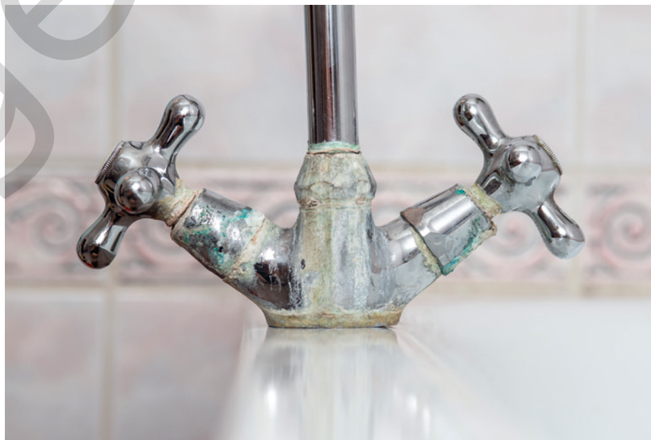
FIGURE 16.2.8 Lime scale around taps is caused by metal ions present in hard water.
