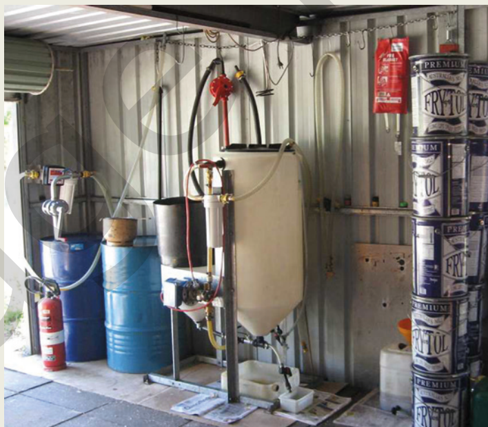
FIGURE 16.4.9 Jonathan Thwaites runs his vehicle on biodiesel made from waste oil in his backyard shed.
